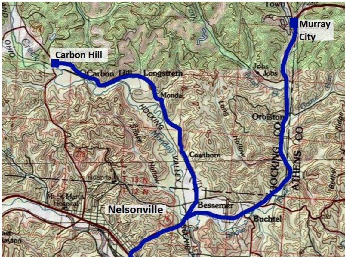
Image 1 - Layout for new sewer collection lines to be installed in Hocking County and connected to the City of Nelsonville in Athens County
